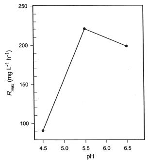
**Figure 3** The effect of medium pH on the maximum degradation rate  $(R_{\text{max}})$  of phenol by immobilized *Pseudomonas putida* ATCC 11172.
