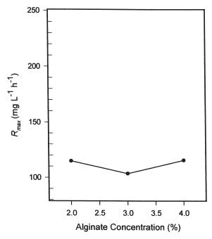
Figure 1 The effect of alginate concentration used in entrapment on the maximum degradation rate  $(R_{max})$  of phenol by immobilized *Pseudomonas* putida ATCC 11172.
