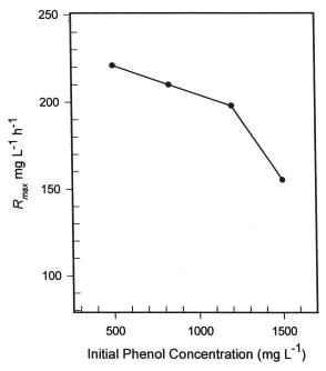
**Figure 5** The effect of initial phenol concentration on the maximum degradation rate  $(R_{\text{max}})$  of phenol by immobilized *Pseudomonas putida* ATCC 11172.
