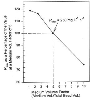
**Figure 6** The effect of the ratio of medium volume to total bead volume on the maximum degradation rate  $(R_{\text{max}})$  of phenol by immobilized *Pseudomonas putida* ATCC 11172.
