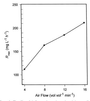
**Figure 4** The effect of air flow on the maximum degradation rate  $(R_{\text{max}})$  of phenol by immobilized *Pseudomonas putida* ATCC 11172.
