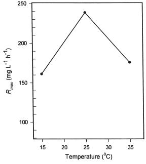
Figure 2 The effect of reaction temperature on the maximum degradation rate  $(R_{\text{max}})$  of phenol by immobilized Pseudomonas putida ATCC 11172.
